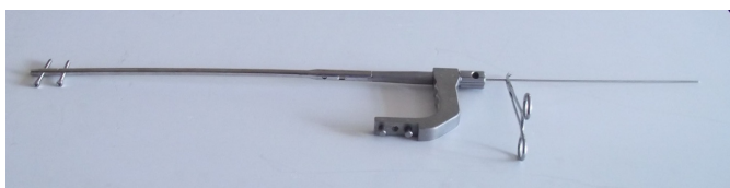
Figure 10: The guide wire cannot advance past the screw. Thus the clamp does not abut on the targeting device.
